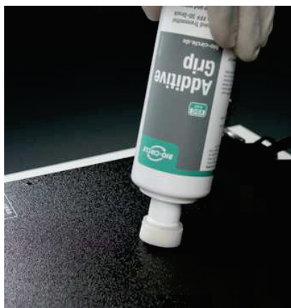
Apply 3D adhesion and release agent to the print bed.
