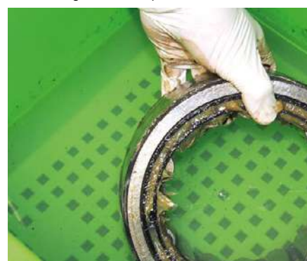
Pre-cleaning of machine parts in the CLEAN BOX
