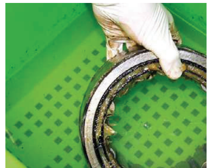
Pre-cleaning of machine parts in the CLEAN BOX
