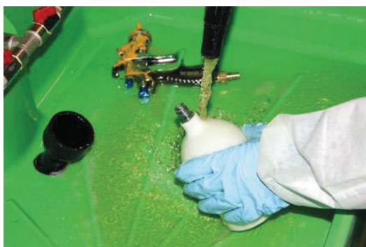
Cleaning spray guns and accessories in the PROLAQ Compact
