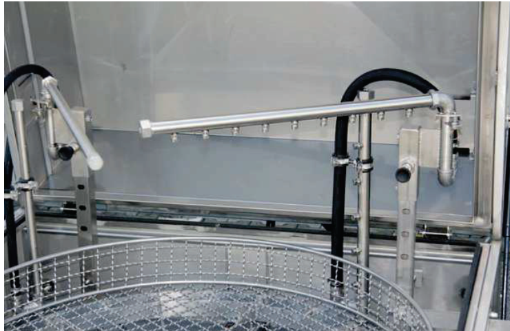
HTW-II Max Eco – Height-adjustable nozzle holder for cleaning and air shower
